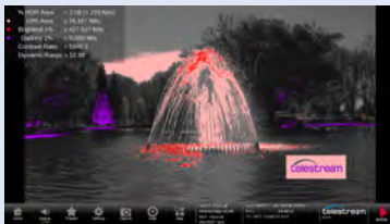
For HDR application determine the Area above the reference white threshold is critical with user thresholds and simple color overlays available in option PROD.
