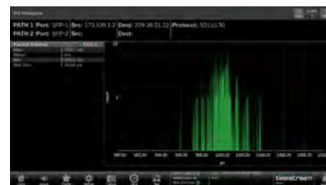
This image shows the PIT Histogram of an Audio Sender being received by PRISM. In this case the Mean packet distribution is 1ms giving an indication of the type of audio being sent.
