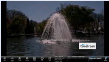
Full screen picture display showing currently selected input signal. In this case, this is camera RAW footage and so it appears to be low contrast and desaturated. For camera RAW and HDR inputs a gamma transfer function and color space conversion can be applied with option PROD.
