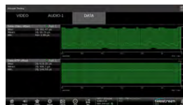
The Data tab shows the Data-Vid offset indicating the relative delay between the data and video stream. In order to realign the signals the delay amount should be applied.
