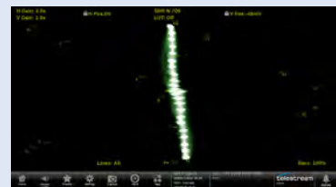
With a camera grey scale chart a deviation in the lower half of the display shows a red offset in the image.
