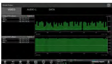
The Video tab shows the Video-PTP offset which is a graphical plot of the Timing displays variation. The Video-RTP offset shows timing of the received signal relative to the embedded RTP time stamp.
