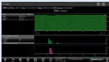
The PIT graphs plots the Packet Interval Time and can show variations within the network. The RTP Sequence Errors shows packet that arrive out of order and whether they can be corrected by the buffer within PRISM.
