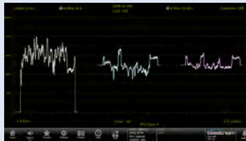
Precise adjustment using Line Select to isolate individual lines within the image.
