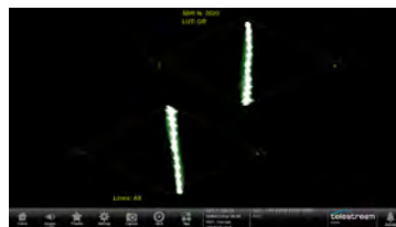
In this example a red offset has been added to the camera greyscale chart cause a deviation in the lower half of the trace.
