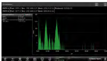
This PIT Histogram shows the characteristics of a Linear Wide Sender that has wide distribution of packets shown by the Min and Max values.
