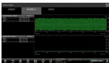
The Audio tab shows the Aud-Video offset that can indicate the amount of delay that must be applied to realign the signals. The Aud-RTP offset shows the timing of the audio stream relative to the embedded RTP time stamps.
