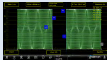
Cursors to measure voltage and time with selectable values of millivolts, percentage, code value and Nits/Stops.
