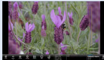
AFD information and graticule can be overlaid within the picture display. Additionally, the user can configure safe area graticules along with a center marker that can be used to help operators compose the image.
