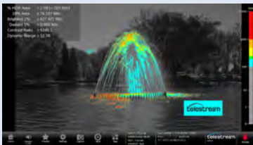
For HDR the False Color overlay can be used to identify the luma level of the signal with user defined limits for each color overlay with option PROD.
